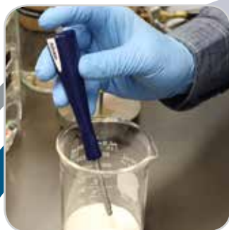
ASAP ® : Atmospheric Solids Analysis Probe
